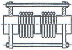
BUTT WELD ARTICULATED WITH TIE RODS
