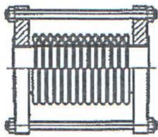
AXIAL WITH FLOATING FLANGES AND TIE RODS
